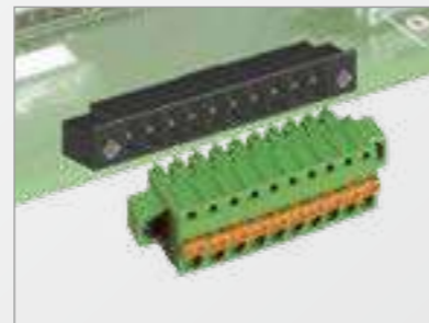
Plug can connect with reflow-solderable sockets
