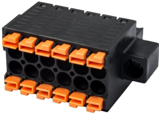
Twin connectors design, the pole number is half of the total connection points. photo shows a 12 connection product, the pole number is 06.
