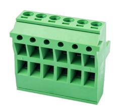
Twin connectors design, the pole number is half of the total connection points, photo shows a 12 connection product, the pole number is 06.
