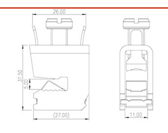
DIN Rail terminal blocks, Busbar terminal blocks
