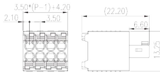
Twin connectors design, the pole number is half of the total connection points. photo shows a 12 connection product, the pole number is 06.
