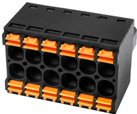
Twin connectors design, the pole number is half of the total connection points. photo shows a 12 connection product, the pole number is 06.
