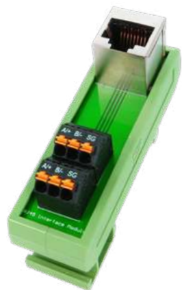
Terminal block 8 pin RJ45 female connector RS485 Interface Wire range (IEC/UL): 0.14 ~ 1.5mm 2 / AWG 28 ~ 16
