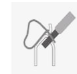
Spring clamp connection
